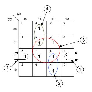
The circled "1"s represent the terms that make up the product terms in the simplified equation. To write the equation for the product terms the row(s) and the columns(s) where the circled group of "1"s are located must be examined.
