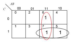
The output equation is Y = AB + AC. As a final step generate a Truth Table using the simplified equations to verify that it is correct.
